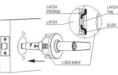
**2B:**Place lock body into position. Make sure that latch prongs engage chassis in housing, and slide engages latch tail.
