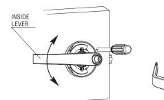
**2D:** Slide inside lever onto spindle and check to see if the rotation is smooth. Adjust the radial clearance between inside spring cage and inside lever if necessary.
