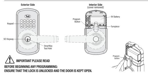
There are two ways to enter the programming mode. First, by pushing the Program Button (shown above in the diagram). A second method is by creating a Programming Code, which allows you to enter the programming mode if you don't have access to the interior of the lock. Please follow the instructions starting in Page 2 or follow the table reference below to begin programming.
