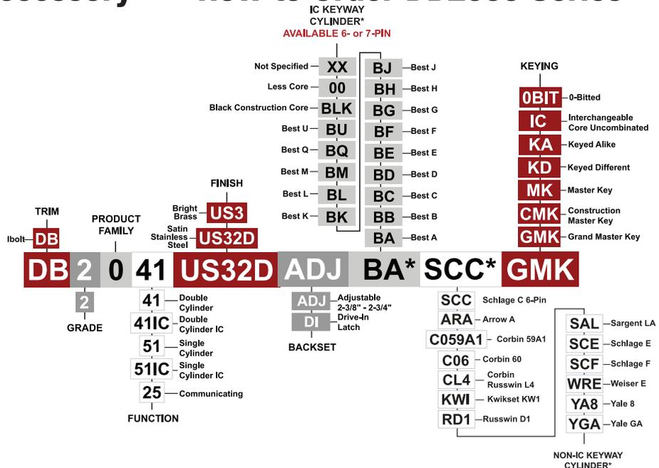
\*Choose one keyway format; either IC KEYWAY CYLINDER or Non-IC KEYWAY CYLINDER
