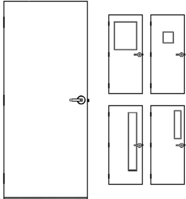
6. All steel glass trim provides a clean, neat, and flush finish with the door surface
