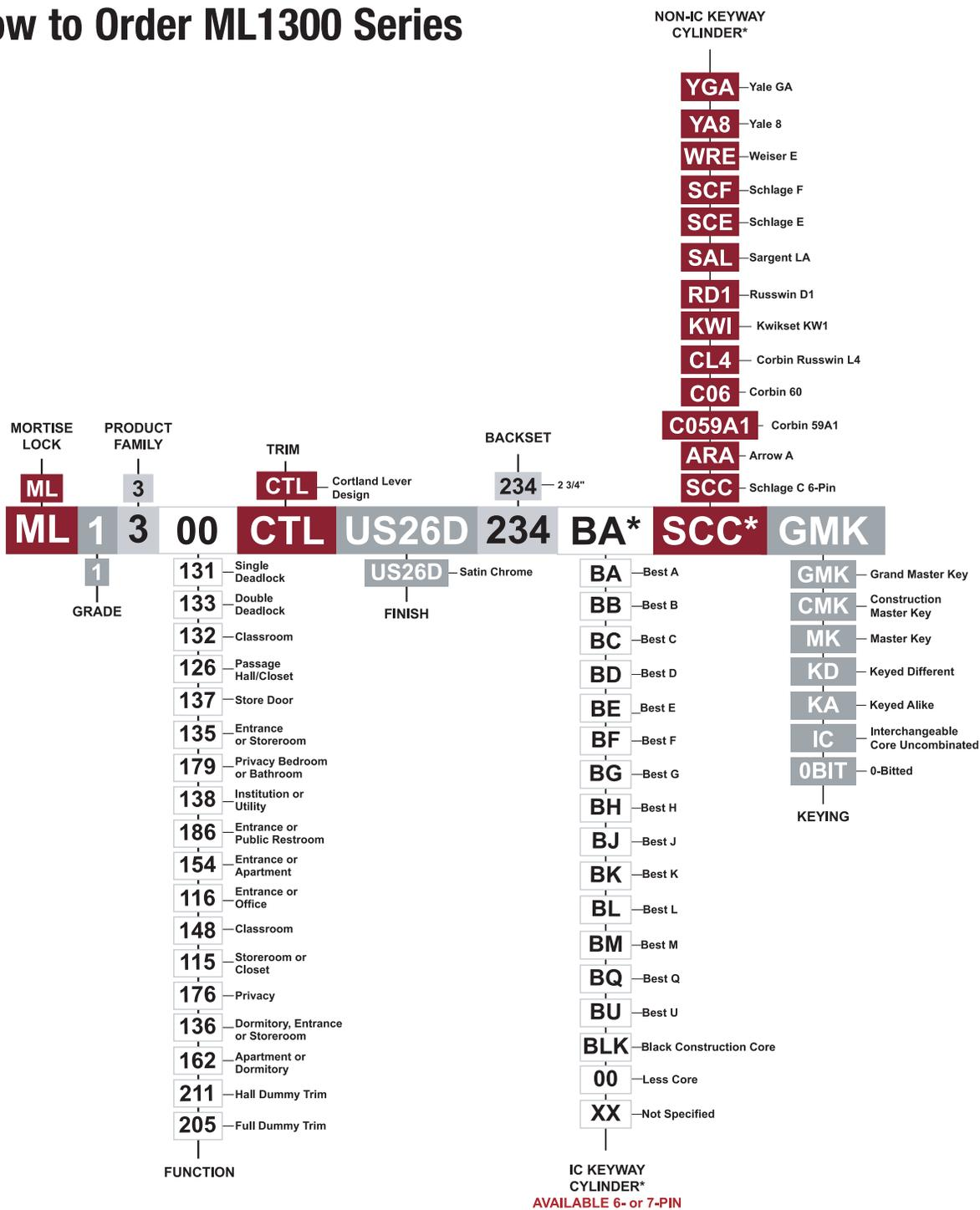
\* Choose one keyway format; either IC KEYWAY CYLINDER or Non-IC KEYWAY CYLINDER
