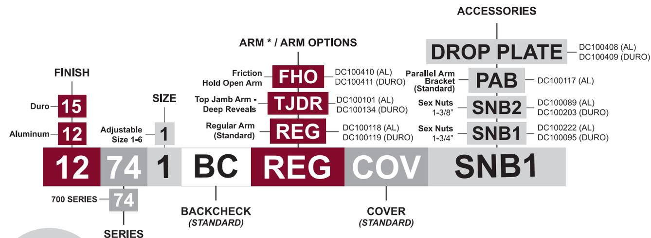
\* TRI-PACK, STANDARD= Regular Arm, Top Jamb Arm 0-3", Parallel Arm Bracket
